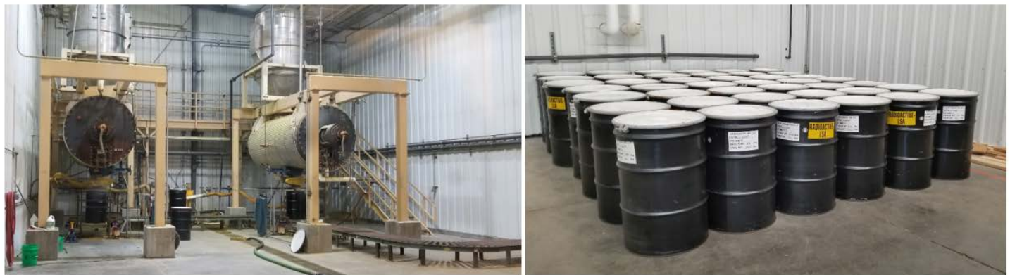
Figure 2: (Left) Lost Creek's Vacuum Dryers allows a dried yellow cake product to be produced at Site. (Right) 42 barrels of ~37.8K lbs dried yellow cake ready to be shipped to ConverDyn to join 233.7k lbs of Inventory.
