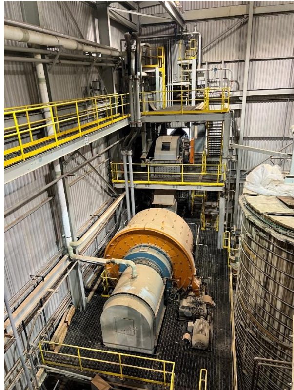
Figure 5: Upper Left: RoM conveyor as it enters the mill; Upper Right: Looking back at RoM conveyor entering mill where ore is gravity-fed to ball mill; Lower Left: Looking at wooden leach tanks from conveyor/ball mill platform – these tanks will be replaced
