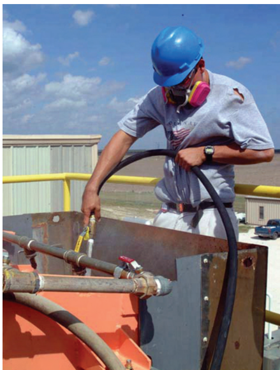
Resin that is delivered to the central plant can also contain formation sand. The resin is washed to remove deleterious elements. Photos courtesy of Uranium Resources.
