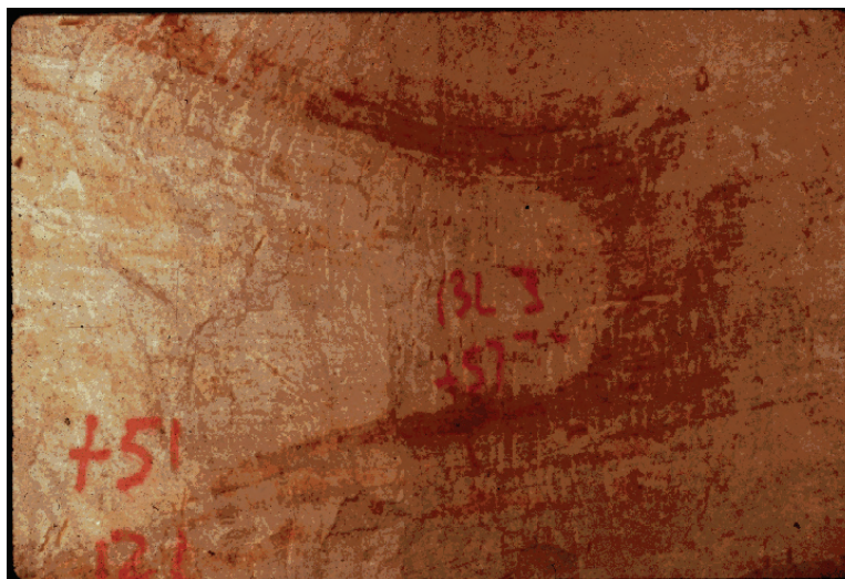
In Wyoming, rollfronts are the most common form of uranium occurrence. These are typically mined through the ISR uranium mining method, also known as solution mining. Above photo shows a rollfront occurrence of uranium minerals (black) in host sandstone, Gas Hills, Wyoming. The sandstone contains reduced forms of minerals on the convex side of the roll-front, while the minerals exist in the oxidized state inside or on the concave side of the roll-front. Photo from C. L. VanAlstine, Office of the U. S. Atomic Energy Commission, Casper, Wyoming, donated to the Wyoming State Geological Survey. Courtesy of WSGS.
