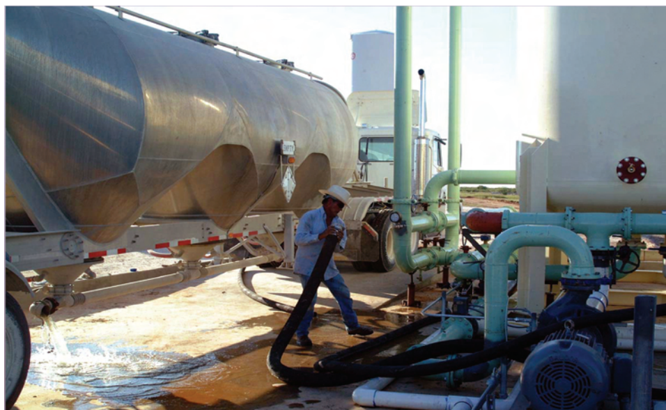
Resin Transfer from Remote Ion Exchange. Photo courtesy of Uranium Resources.
