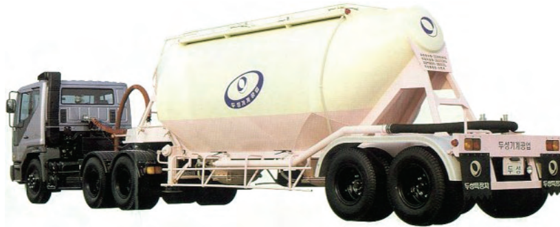
Uranium Resources buys new bulk cement trailers, such as the one above, and modifies these for trucking the uranium-loaded resin. These specially designed transport systems are generally used for oil, chemicals, bulk cement, grains/flour and fly ash. Courtesy of Elemans Corporation.
