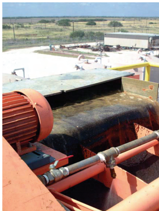
Resin that is delivered to the central plant can also contain formation sand. The resin is washed to remove deleterious elements. Photos courtesy of Uranium Resources.
