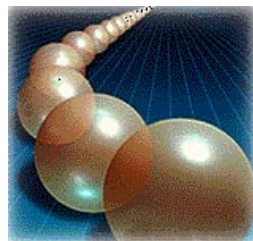
Millions of small polymer resin beads adsorb the uranium in solution.
