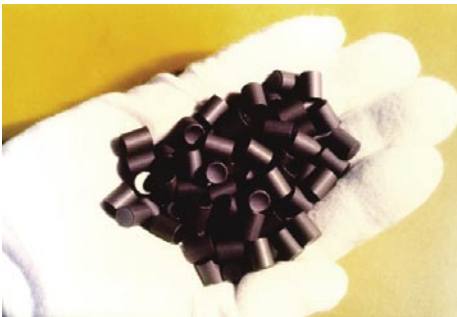
Two uranium pellets produce enough energy to supply, for an entire month, an average four-person household.
